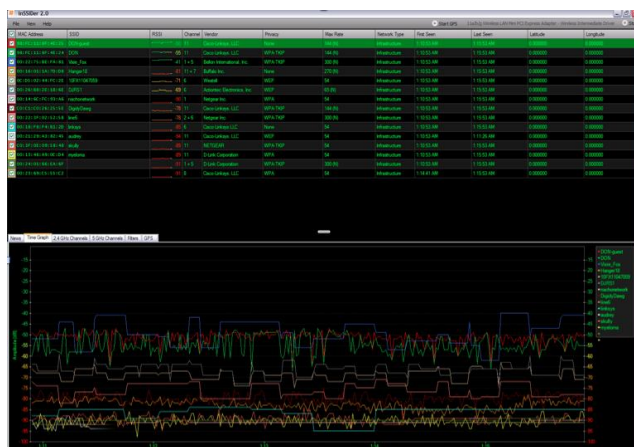
Fig.2.3 The amplitude of signals varies for different AP's.
